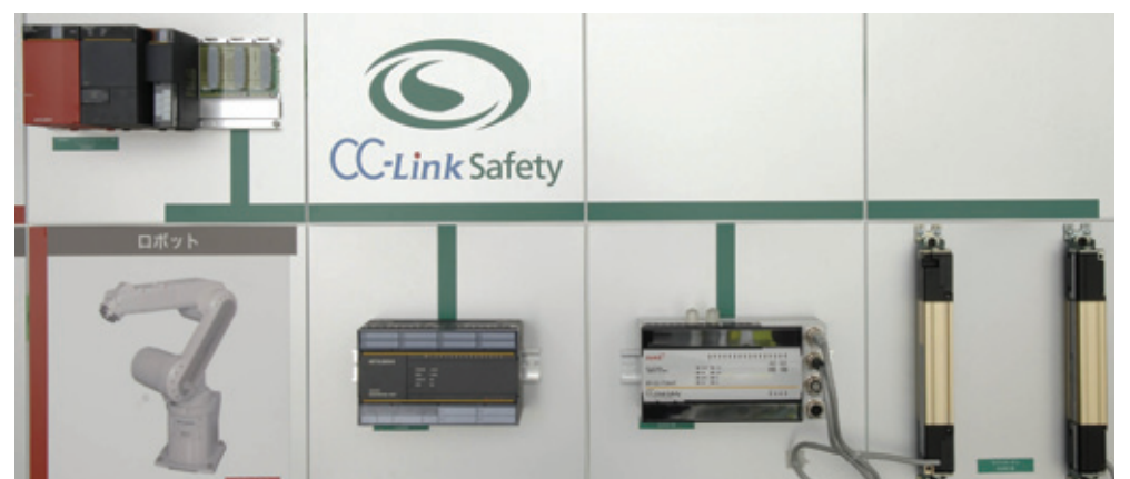
Mitsubishi Electric Corporation Safety PLC MELSEC-QS Series Sunx Limited Light Curtain remote I/O unit (available soon)
