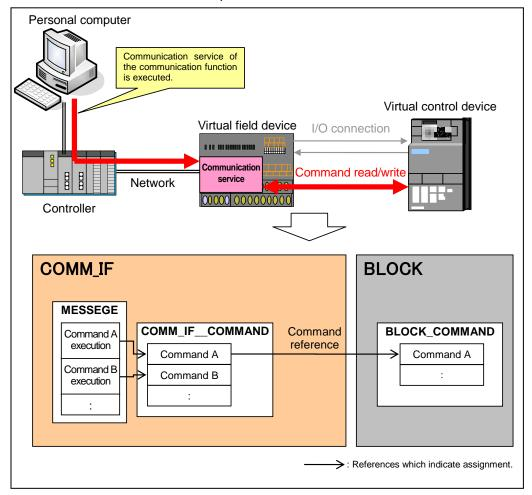
Figure 4.5-1 Reference Specifications Example of the COMM\_IF\_COMMAND Part
