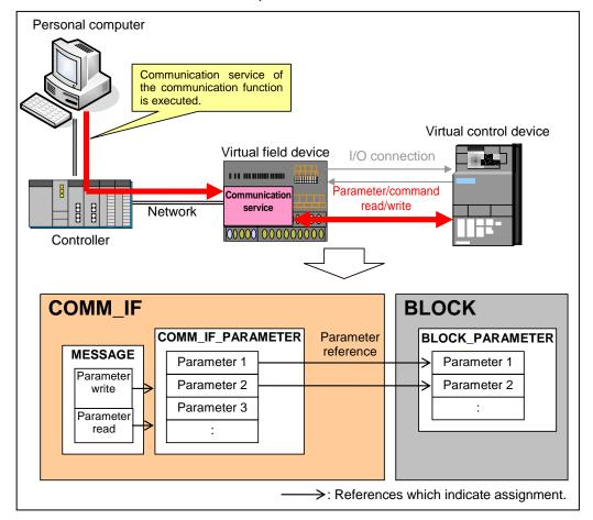
Figure 4.4-1 Reference Specifications Example of the COMM\_IF\_PARAMETER Part
