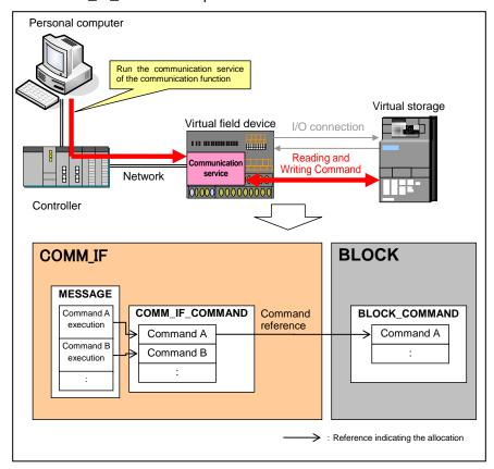
Figure 5.5-1 Reference Specifications Example of the BLOCK COMMAND Part
