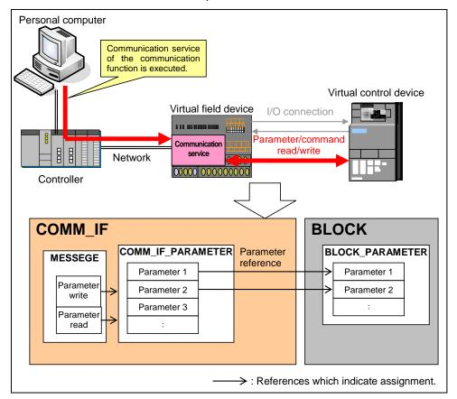
Figure 5.4-1 Reference Specifications Example of the BLOCK PARAMETER Part
