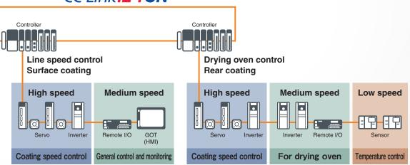
Cyclic communication is enabled by suppressing the effect of each device station's performance response.
