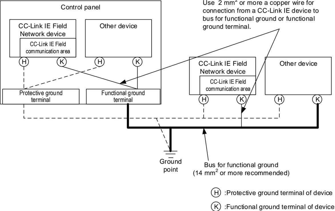
Figure 13 Wiring Example of Shared Grounding
