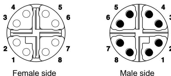
**Figure 6 M12 (X-coding) Connector**
