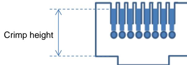
Figure 15 Crimp Height of RJ45 Connector (Plug)
