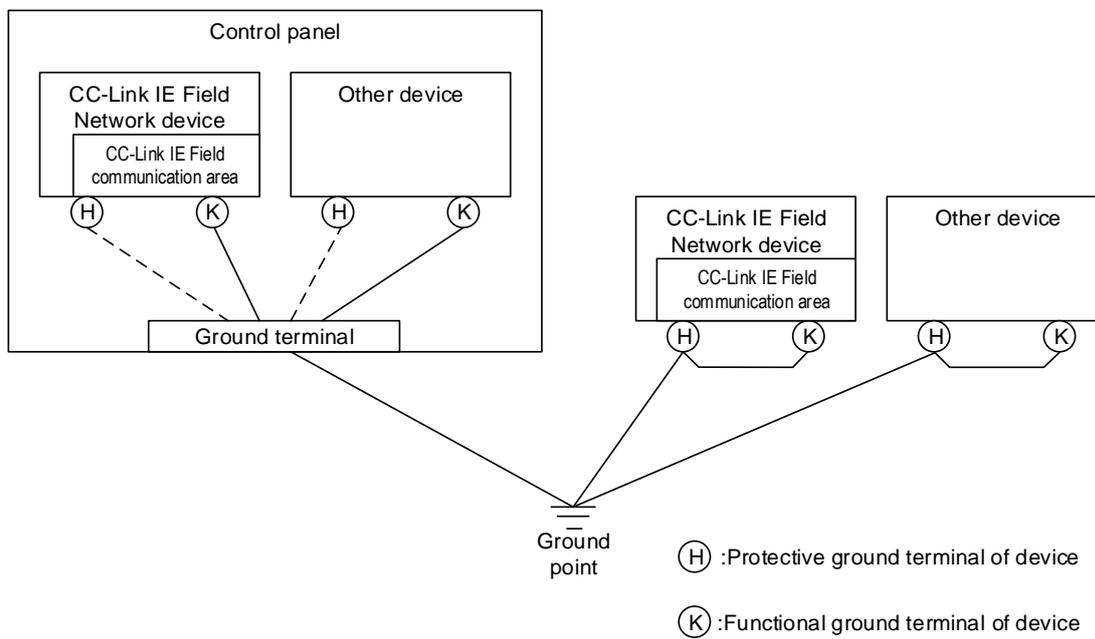
**Figure 12 Example of Common Grounding**
