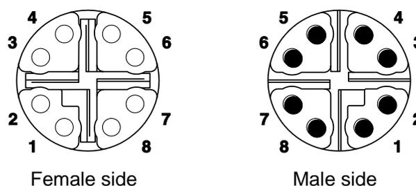
**Figure 6 M12 (X-coding) Connector**
