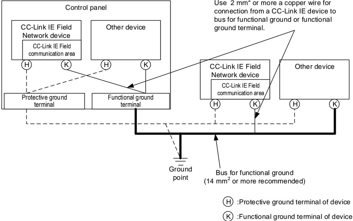
Figure 13 Wiring Example of Shared Grounding
