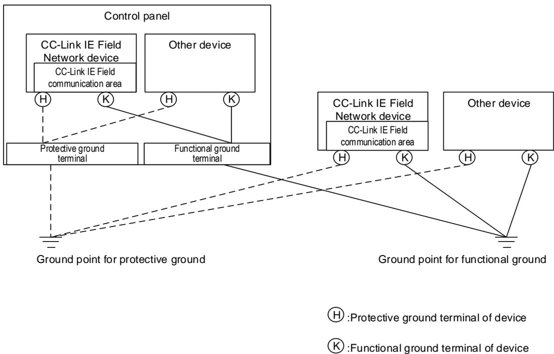
**Figure 10 Example of Independent Grounding**
