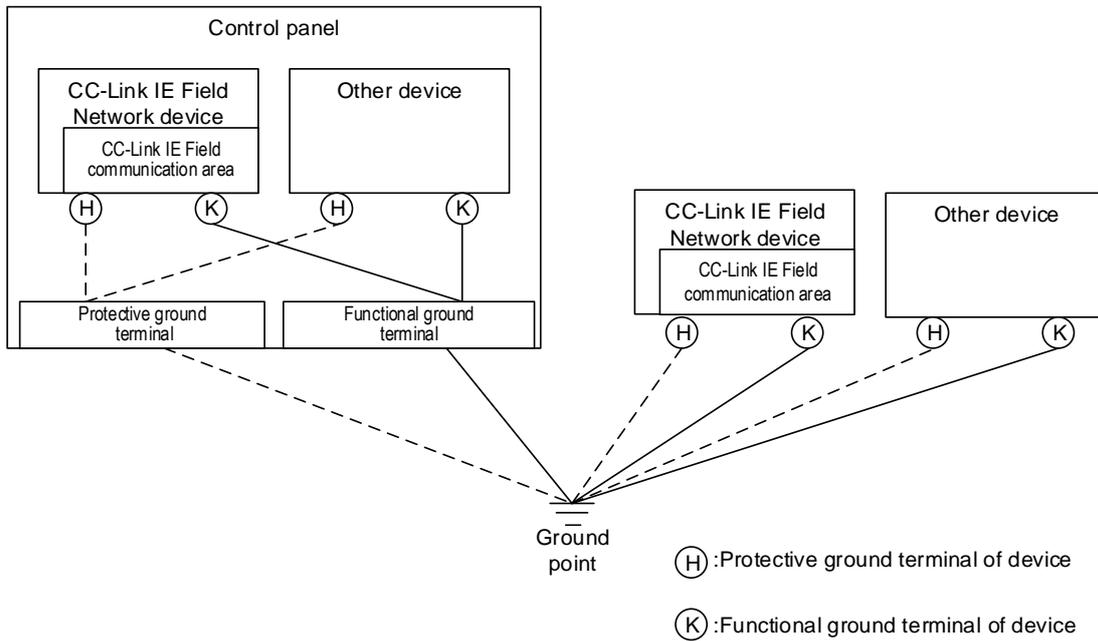
**Figure 11 Example of Shared Grounding**
