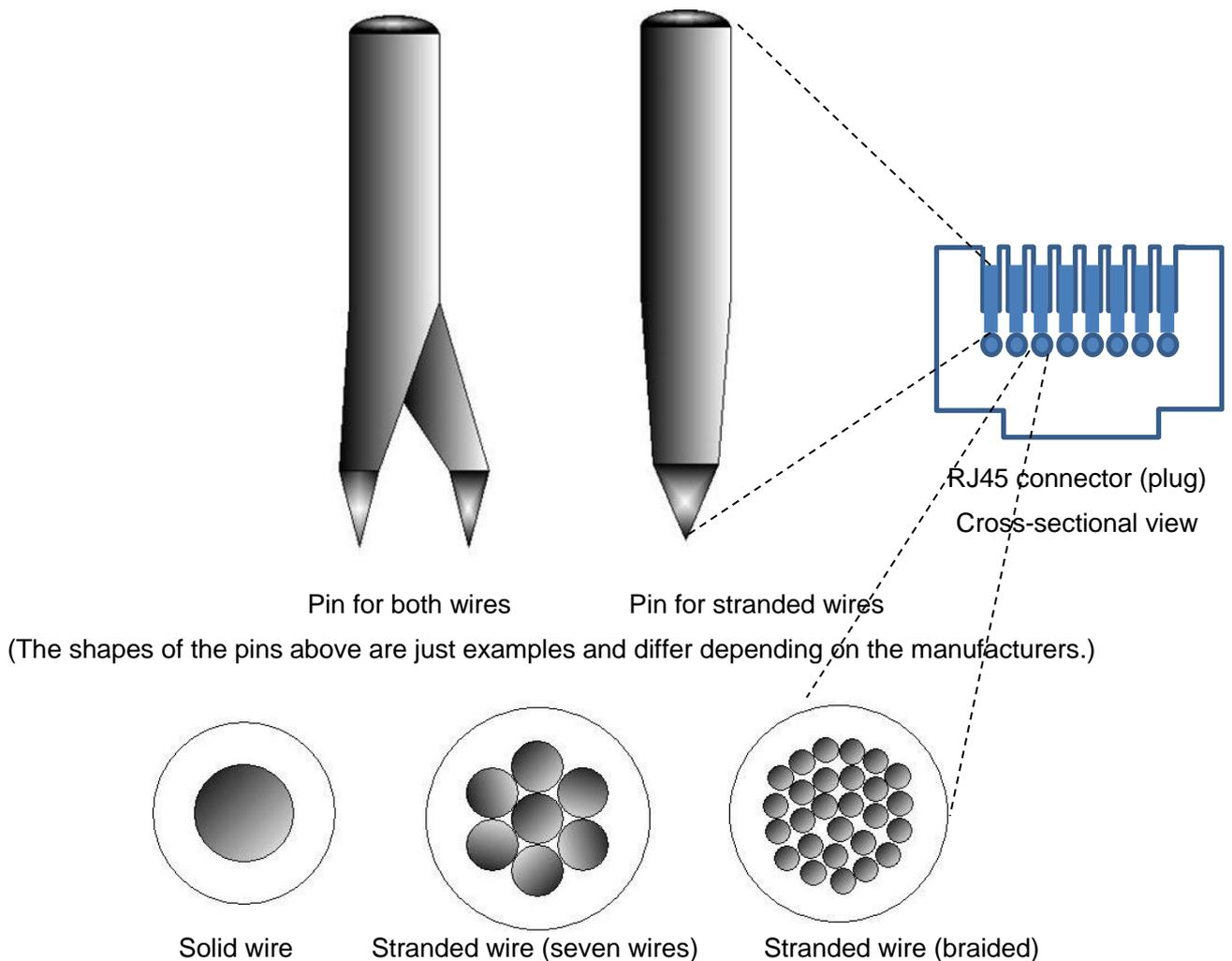
Figure 14 Pin Shape Examples of RJ45 Connector and Wire Types
