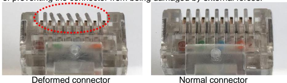
Figure 17 Example of a Deformed RJ45 Connector
