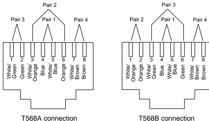
**Figure 5 Connection Method with the RJ45 Connector (Plug)**
