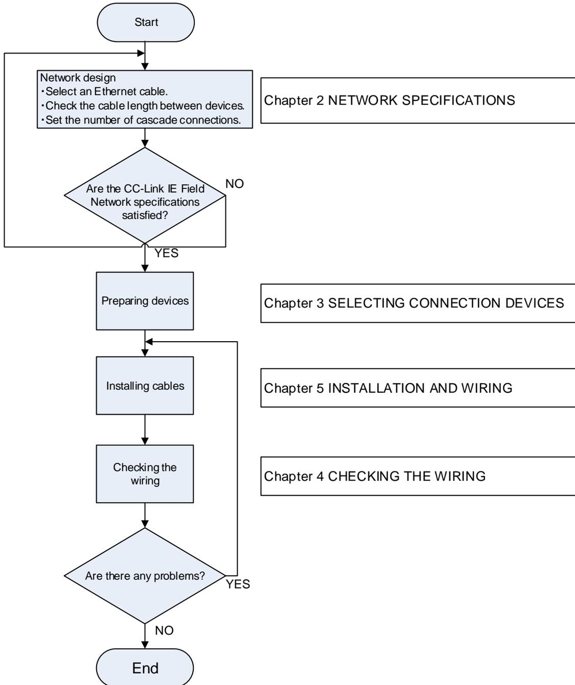
**Figure 1 Network Configuration Procedure**
