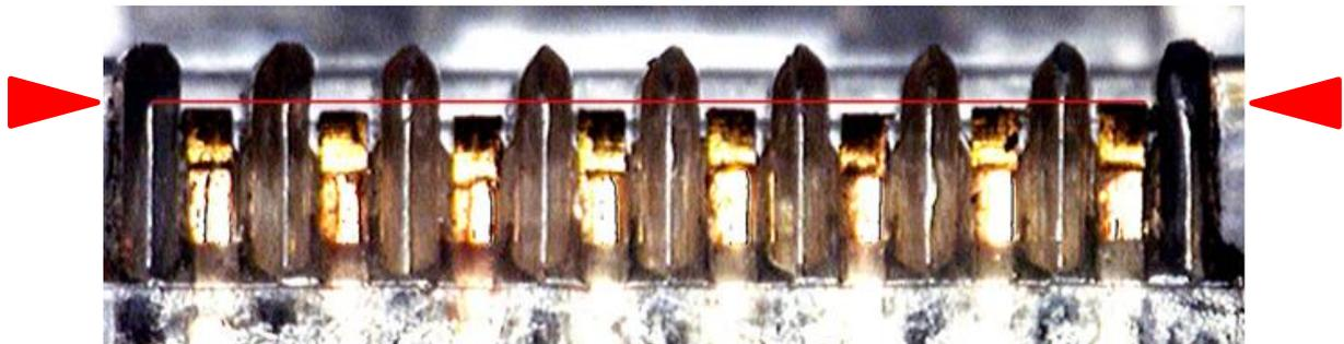
Figure 16 Uneven Crimp Height Example of RJ45 Connector (Plug) with Crimp-Type Contacts
