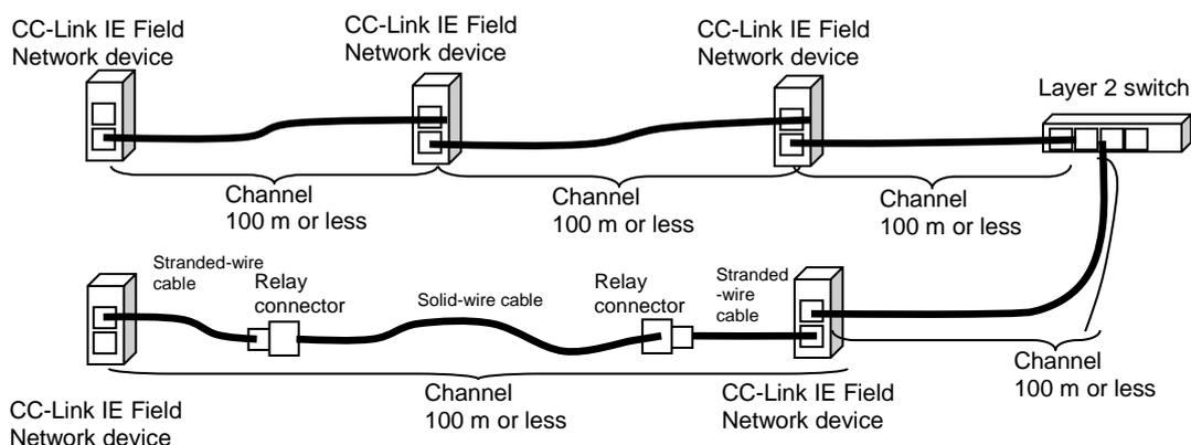
**Figure 4 Wiring Length**
