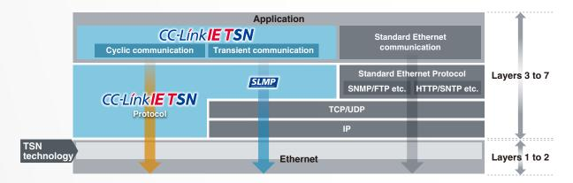
TSN consists of multiple international standards. The major standards are IEEE802.1AS (which defines the time synchronization method) and IEEE802.1Qbv (which defines the time sharing method). Combining these to the Ethernet standard enables punctuality, ensuring transmission within a given period of time, and mixed implementation with other communication protocols.
