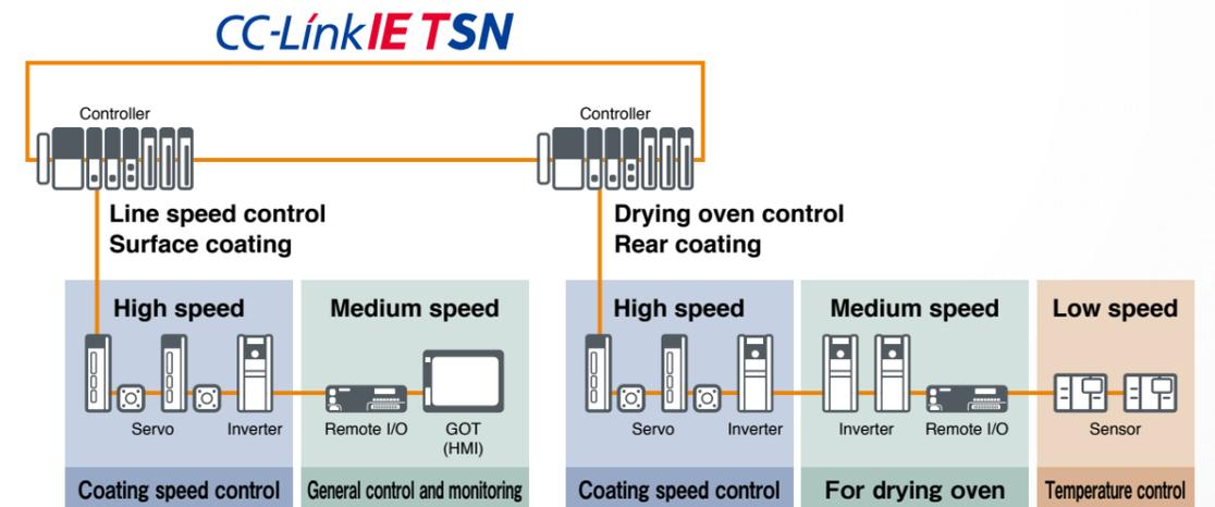
Cyclic communication is enabled by suppressing the effect of each slave station's performance response.
