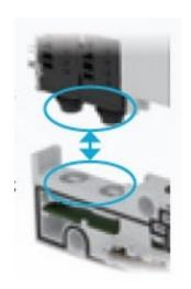
Additional actuators can be connected by plugging in the wiring.
